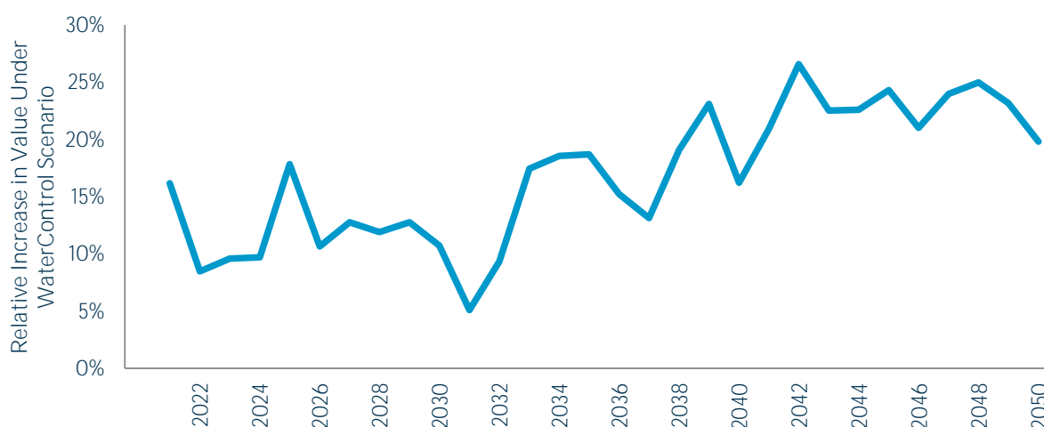
Figure 38. Modelled relative increase in value of energy through the increase in controllability of the Derwent. This could be achieved through selective improvement of controllability of the system, such as redeveloping the Tarraleah scheme to be more controllable
