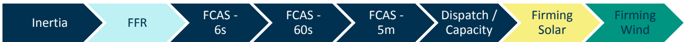
Figure 25. Time requirements for energy supply, highlighting newer requirements. Fast frequency response (FFR), also sometimes called synthetic inertia, will provide some measure of resilience as many of the major inertia providing stations retire. Solar will need firming over several hours and wind will need firming for periods up to days
