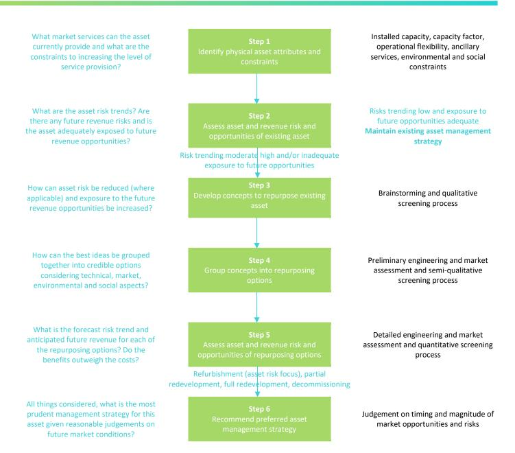
Figure 1: Framework for repurposing existing hydropower assets for the future electricity market
