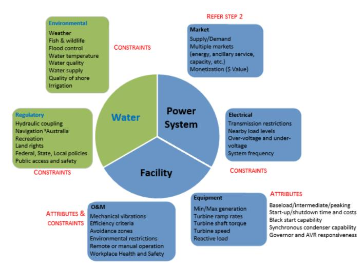
Figure 3: Complexity of operational factors for hydro plants (EPRI, May 2017)
