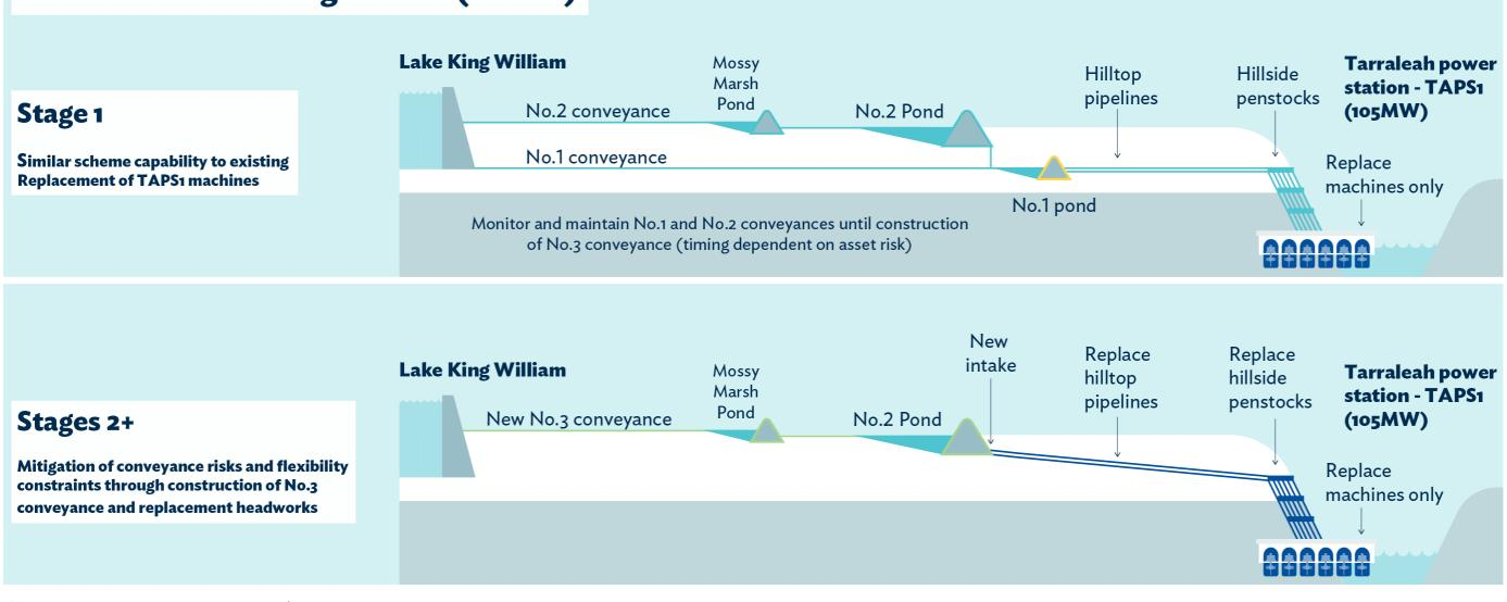
Figure 15: Maintain existing station option diagram
