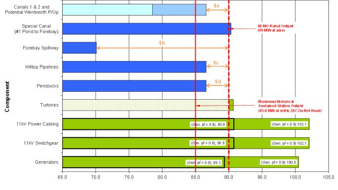
Station Output (MW at wire)
