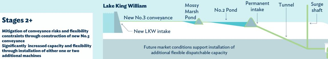
Figure 18: New 4 machine station option diagram
