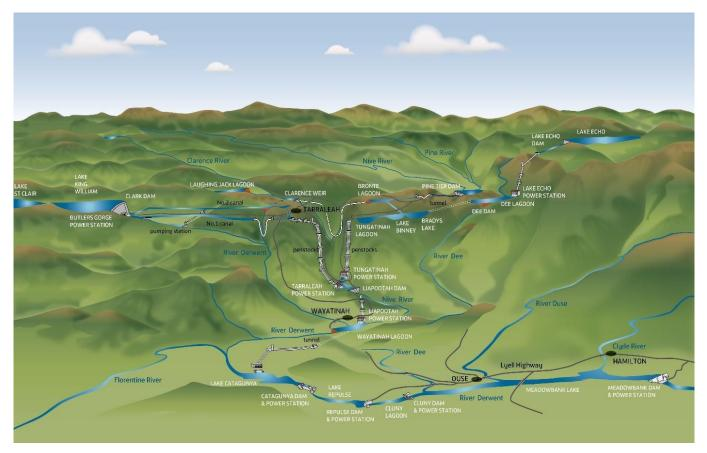
Figure 8: Derwent hydropower scheme diagram
