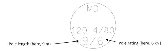
Figure 1: Hydro Tasmania timber pole identification tag
