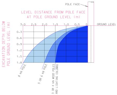
Figure 2: Temporary excavation limits when working near Hydro Tasmania's power poles
