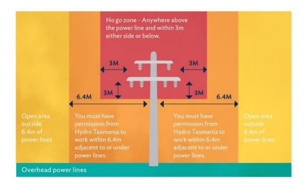
Figure 3: Working near overhead power lines
