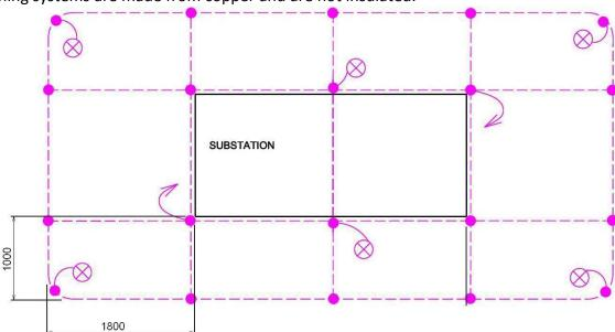
Earthing systems are made from copper and are not insulated.
