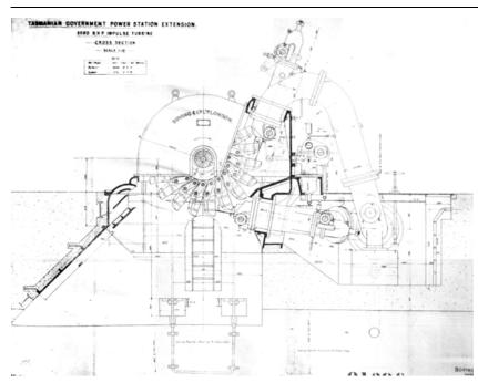
Figure 3.7 Plan of two jet Turbine.
