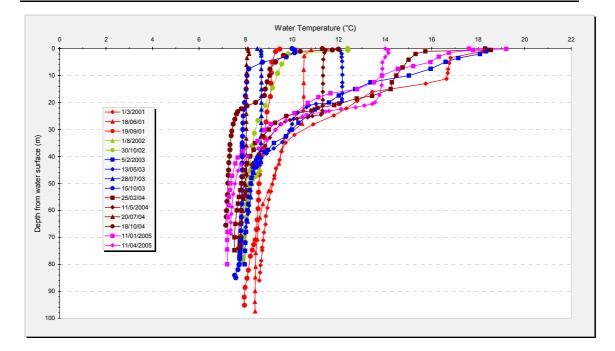
Figure 11.1. Temperature profiles from the Lake Gordon near the intake.
