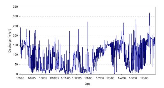
Figure 2.8. Flow recorded (hourly data) at site 65 (Gordon above Denison), from July 2005 to June 2006.
