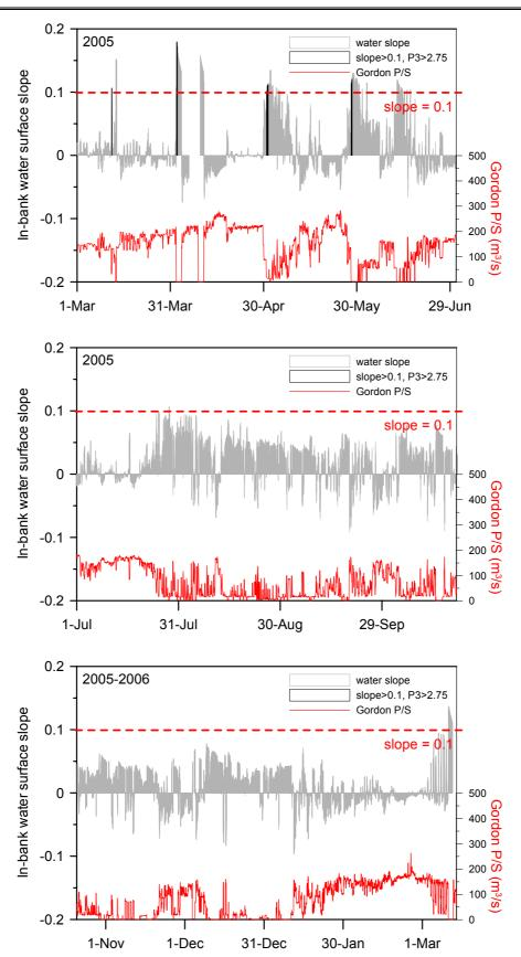
Figure 4.4. In–bank water surface slopes (upper) and discharge from Gordon Power Station (lower). Periods when water slopes exceed 0.1 and water level at probe 3 exceeds 2.75m are highlighted in black.
