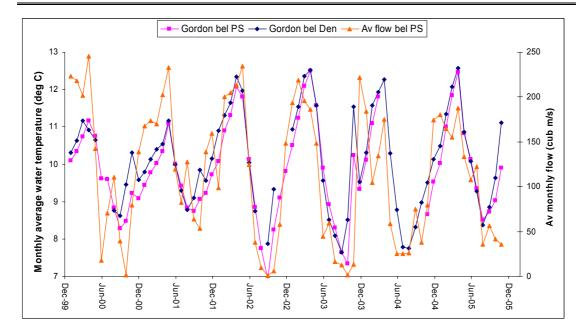
Figure 11.5. Average monthly flow rates superimposed on the water temperature curves.
