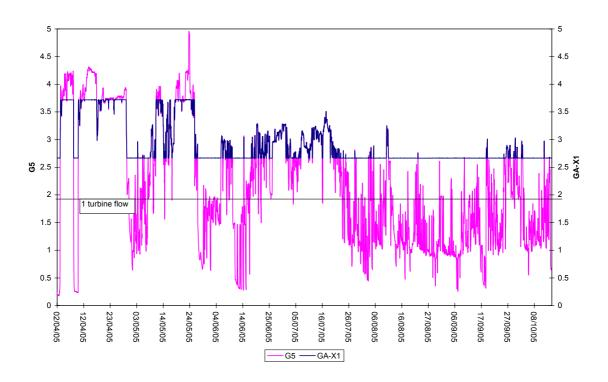
Figure 5.5. GA–X1 water level recorder with water levels from site 72 (G5) for comparison for the period of 2 April–15 October 2005. Data in metres above arbitrary zero datum.
