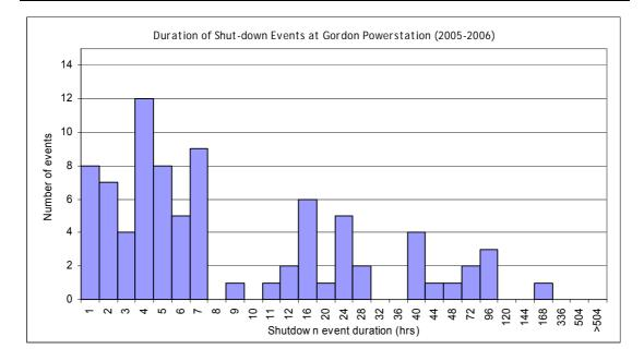
Figure 2.6. Frequency and duration of zero discharge (shut–down) events recorded for the Gordon Power Station during 2005–06.
