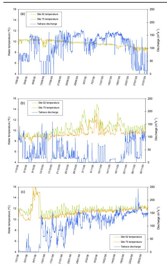
Figure 3.6. Water temperatures at sites 75 (2 km downstream) and 62 (15 km downstream) and corresponding tailrace discharge for (a) June–July 2005, (b) October–November 2005 and (c) January–February 2006.
