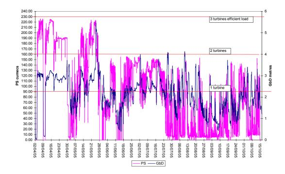
Figure 5.2. Power station output in cumecs together with the flow level data from the Gordon below Denison (site 62) gauging station for the period 2 April–15 October 2005.
