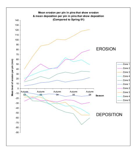
Figure 11.14. Erosion pin results grouped by pins showing erosion and pins showing deposition for each zone. The derivation and analysis of this graph is discussed in more detail in the Gordon Geomorphology chapter.
