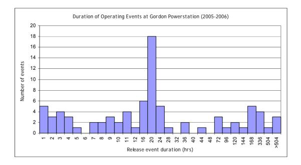
Figure 2.7. Frequency and duration of operating events (discharge > 3 m<sup>3</sup> s<sup>-1</sup>) recorded for the Gordon Power Station during 2004–05.
