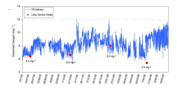
Figure 3.7. Dissolved oxygen values recorded at the power station tailrace from July 2004–June 2005. Spot values represent the measurement of dissolved oxygen at the Lake Gordon intake site that correspond to the level of the power station intake.
