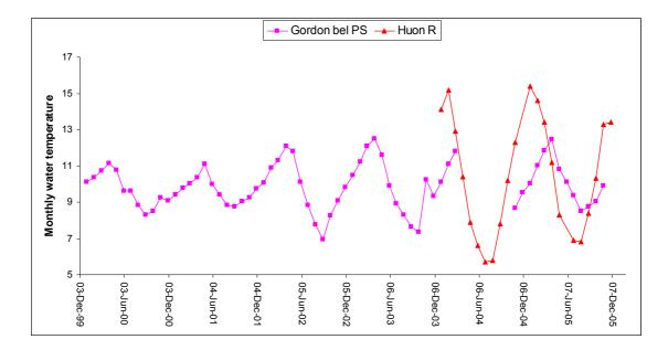
Figure 11.2. The monthly average water temperatures at the Gordon River below the power station, and the unregulated Huon River at Judbury.
