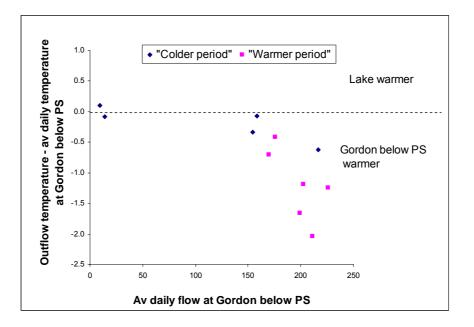
Figure 11.6. Difference between water temperatures at the Gordon below power station monitoring site and water temperature in Lake Gordon at the depth of the intake (254m) compared with flow rates from the power station.
