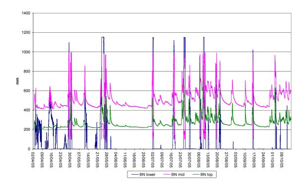
Figure 5.3. Bill Neilson Cave water level recorder data (cave stream only: BN cave top; cave stream and Gordon river water backflooding: BN cave mid; Gordon River backflooding only: BN cave lower) for the period of 2 April–15 October 2005.
