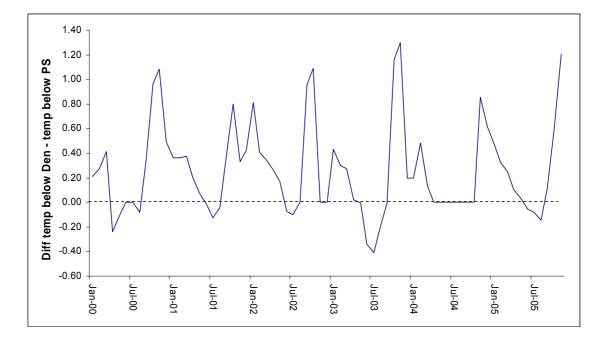
Figure 11.4. Difference in average monthly water temperature at the Gordon below Denison site and the Gordon below power station site. Negative values indicate water below power station is colder than water below Denison.
