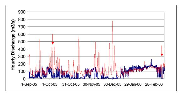
Figure 4.2. Power station discharge, 1 March 2005–15 March 2006. Arrows indicate sampling dates. Blue line shows discharge from the Gordon Power Station, red line shows discharge at the Gordon above Franklin gauging site.
