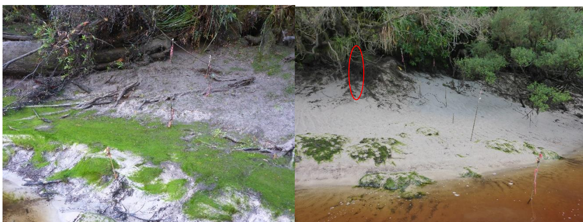
Figure 3-22: Site 3C (left), showing pins 3C4 located on the flat lying lower bank, and pin 3C5 on the bank toe in an area being scoured (right) Site 3E showing location of pin 3E2 at edge of root-mat.
